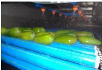
Figure 28: HWT treatment system
