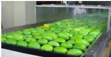
Figure 27: Mangoes washing system
